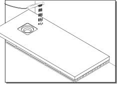
3. Apply PU/MS putty or silicone between the tray and the base to attach it. Apply a silicone bead to the joins of the shower tray with the wall and the floor.
