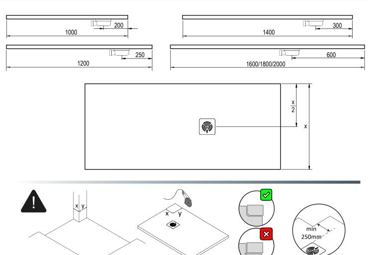
1. Create an even support surface for the whole dimension using a levelling mortar and leave it to set for the amount of time indicated by the manufacturer.
