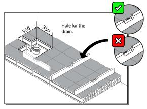
Ensure that the falling water and pipes are not aligned so that drainage capacity is not lost.
