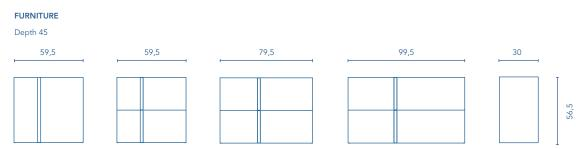
The compositions of 120 are combined with 2 units of 60 The 90 measurements are based on the 60 and 30 modules.
