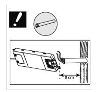
\*Note 1: The length of the power supply cables must not exceed 8 cm.
